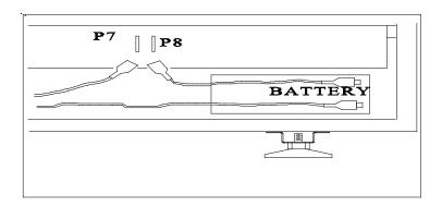
Plug in the two connectors as illustrated. The display on the console will now read ALARM ACTIVATED ENTER PIN NUMBER.
