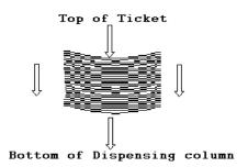
A wide opening at the top of each column allows you to enter stacks of tickets. Grasp a manageable stack of tickets. Slide the stack down the chute. Continue to load tickets until the column is full.
